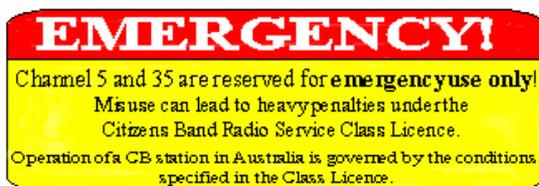
Sample label for UHF equipment (not necessarily to size or scale). Final sticker should be designed to fit on the equipment whilst remaining legible.
